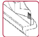
Sharpening of back and side surfaces
